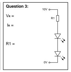
The next 3 circuits are a bit tricky - so think carefully about the voltages and apply principles you have learnt. Again, VF = 3 volts,
