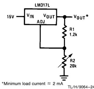
**50 mA Constant Current Battery Charger for Nickel-Cadmium Batteries**
