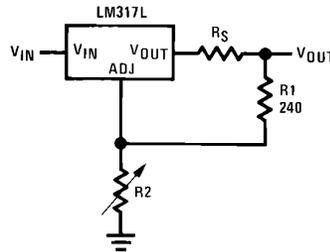
FIGURE 2. Regulator with Line Resistance in Output Lead
