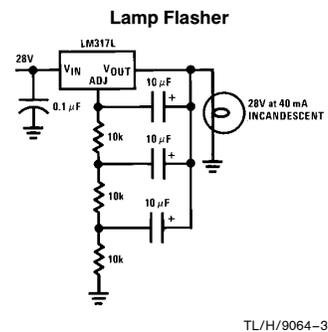
Output rate—4 flashes per second at 10% duty cycle
